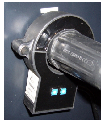
Shunt fitted to negative or positive terminal on the welding machine.
